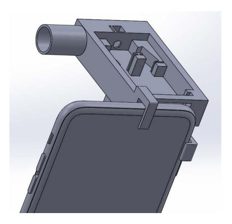
(design the holder and attached the model of the iphone in the solidwork)
